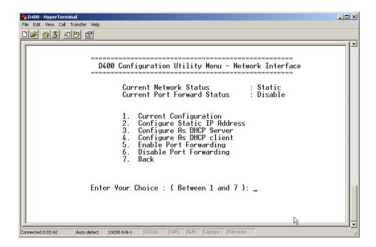
3. Type 2 and press Enter to select 2. Configure Static IP Address.
